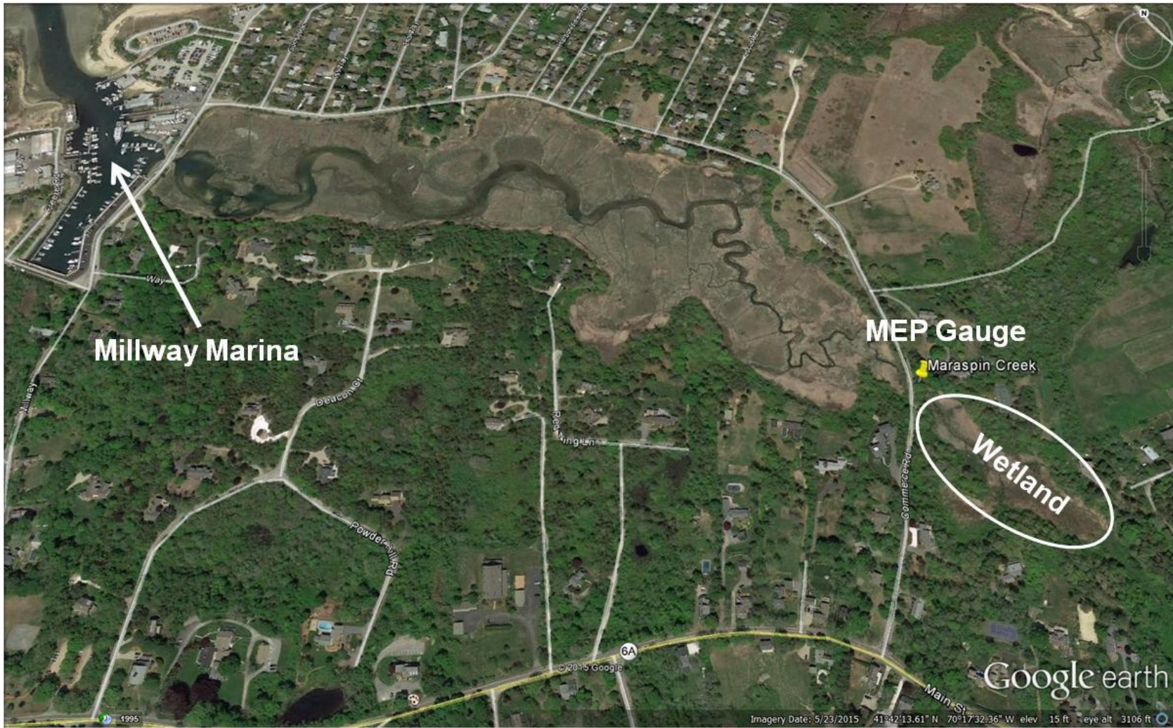
Figure IV-13. Location of MEP stream gauge (yellow symbol) for measuring flow and nitrogen load in Maraspin Creek. The Maraspin Creek salt marsh receives groundwater flow from surrounding residential upland as well as a small wetland and agricultural area up-gradient of the MEP gauge. The creek discharges to the down gradient estuarine receiving waters of the Barnstable Harbor-Millway.
