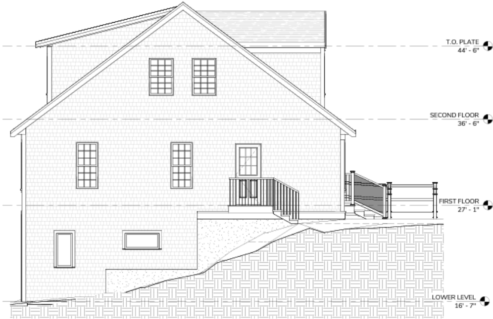
3 EXISTING LEFT SIDE ELEVATION 1/4" = 1'-0"
