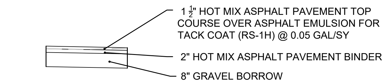
PROPOSED HOT MIX ASPHALT DRIVEWAY
