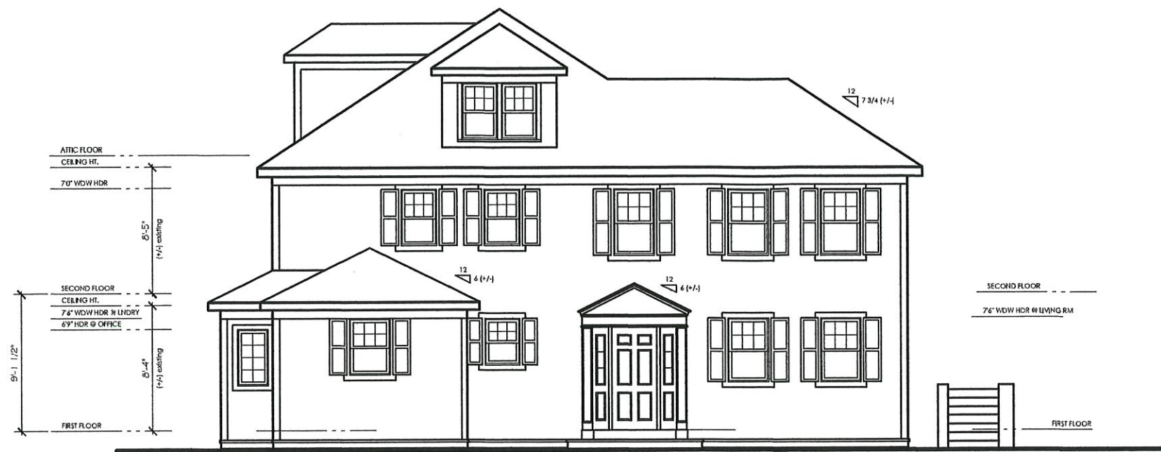
EXISTING WEST ELEVATION 1/4" = 1'-0"
