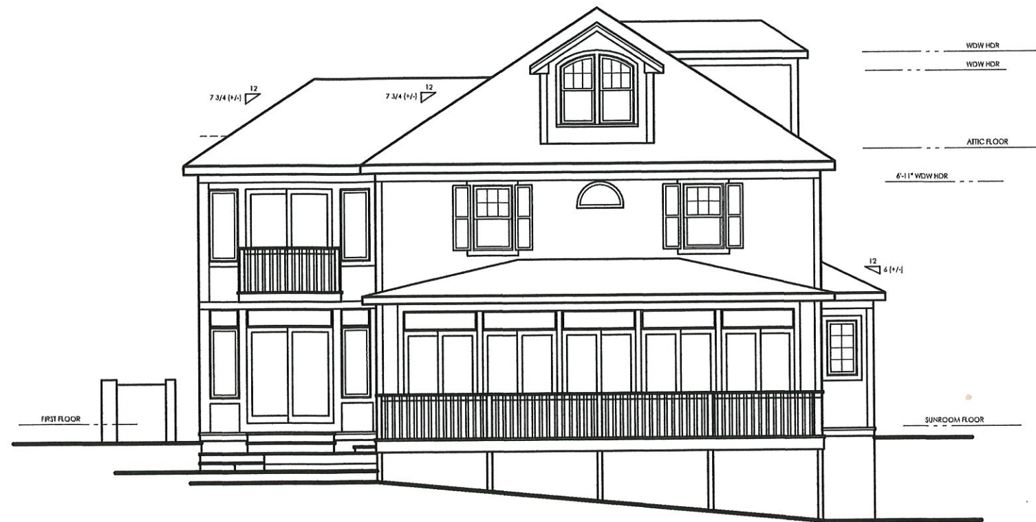
EXISTING EAST ELEVATION 1/4" = 1'-0"
